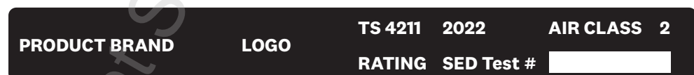
Example 3 – Type of classification TS 4211:2022, exposure rating SED (test report number to be added by window manufacturer or supplier), air permeability class 2
