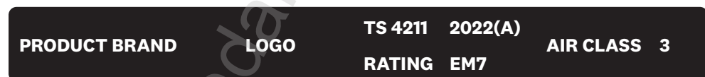
Example 2 – Type of classification TS 4211:2022(A), exposure rating EM7, air permeability class 3
