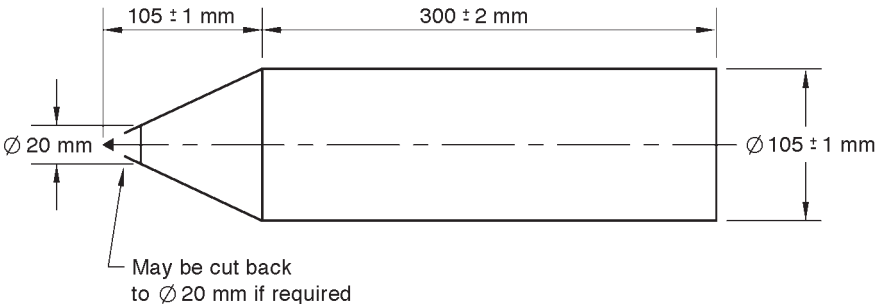
Figure C1 – Test object for testing openings and other components
