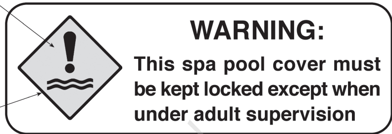
Figure G3 – Spa cover warning signage
