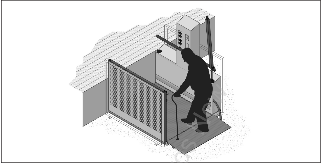
Figure 15 – Example of an open platform lift with travel distance less than 1 m
