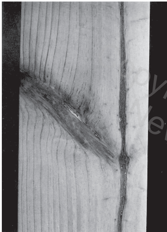
Fig. 7 KNOTS – PARTIALLY INTERGROWN SPIKE KNOT AND PITH
