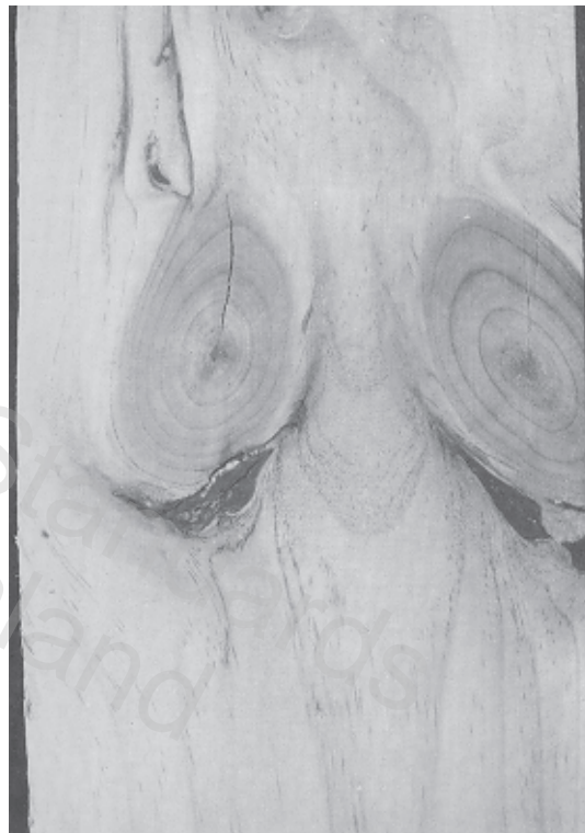
Fig. 6 KNOTS – PARTIALLY INTERGROWN KNOT AND ASSOCIATED BARK POCKET
