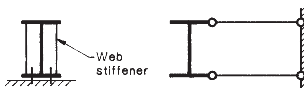
(a) Critical flange lateral restraint, effective twist restraint
