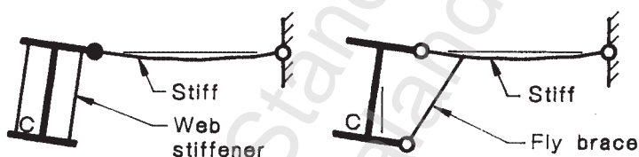
(c) Non-critical flange lateral restraint, effective twist restraint
