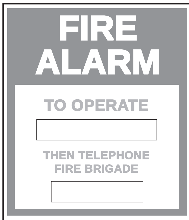
Figure E1 – Notice to be displayed on, or adjacent to, each manual call point
