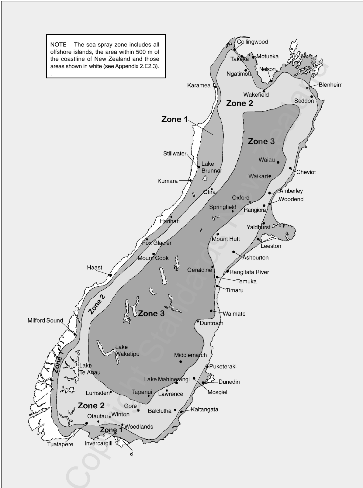
Figure 2.E1 – Corrosion zone map (continued)
