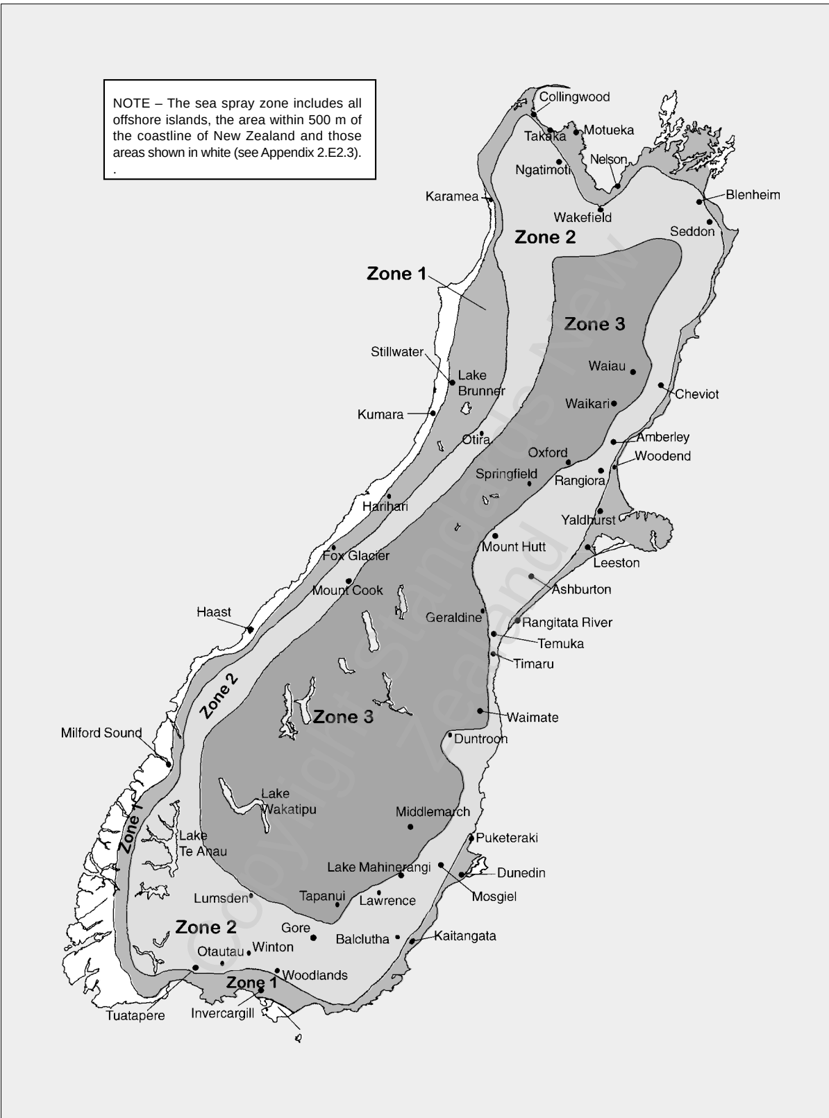
Figure 2.E1 – Corrosion zone map (continued)
