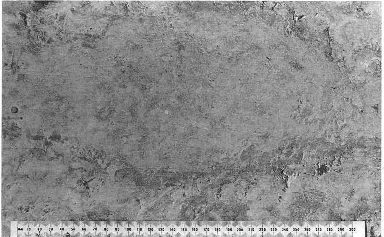
Fig. 7 PHOTOGRAPH OF TYPICAL SURFACE ILLUSTRATING CLASS F3 OFF-THE-FORM FINISH
