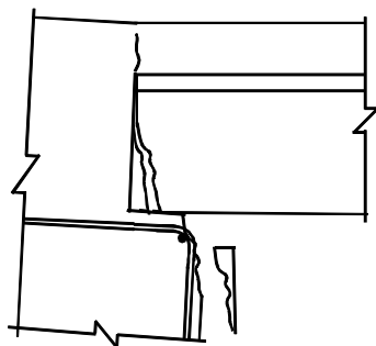
Figure C18.9 – Damage to support ledge and precast unit due to friction and rotation
